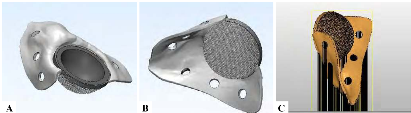
Figure 2. 3D graphic representation of the prosthesis. A. & B. Isometric view of the prosthetic component; C. Positioning of the prosthetic during the process of slicing that lead to the finished product.
